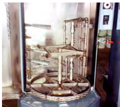
(3) Model 1212 12" (305mm) Standard Air Knives perform the drying cycle in this parts washer.
