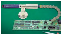
Electronic components stay cool during a soldering operation.
