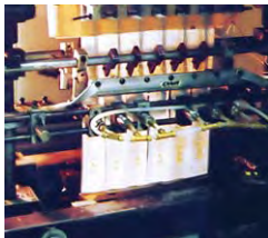
A Model 1212 12" (305mm) Standard Air Knife opens mustard packets prior to fill.
